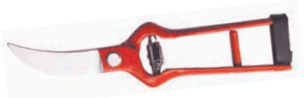
PS33602 Drop forged pruning shears Available size: 7"(180mm) Material: whole-piece drop forged 55# high carbon steel Hardness: whole-piece heat treatment with hardness 52-54HRC Surface: Fully machine grinding Handle: red powder coated
