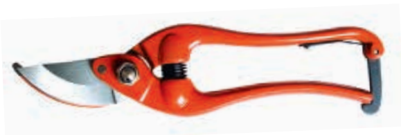
PS33603 Drop forged by-pass pruning shears Available size: 8"(200mm), 9"(230mm) Material: drop forged 55# high carbon steel body, 65# MN steel changeable blade Hardness: whole-piece heat treatment with hardness 52-54HRC on body, 54-56HRC on changeable blade Surface: machine grinding on changeable blade Handle: red powder coated.
