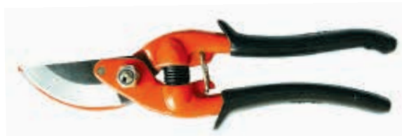
PS33605 Drop forged by-pass pruning shears Available size: 8"(200mm), 9"(230mm) Material: drop forged 55# high carbon steel body, 65#MN steel changeable blade Hardness: whole-piece heat treatment with hardness 52-54HRC on body, 54-56HRC on changeable blade Surface: black finished on changeable blade, red powder coated on body Handle: soft black PVC grips
