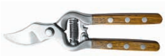
PS41011 Drop forged by-pass pruning shears Avilable size: 8" Material: whole-piece forged stainless steel Hardness: whole-piece heat treatment with hardness 51-53HRC Surface: Mirror polished Handle: ash wooden handle with fully polished
