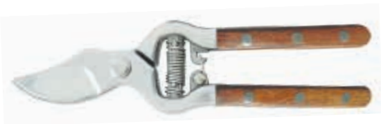
PS41013 Drop Forged by-pass pruning shears Available size: 8" Material: whole-piece drop forged stainless steel Hardness: whole-piece heat treatment with hardness 51-53HRC Surface: mirror polished Handle: wooden with fully polished
