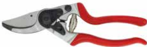
PS113303 Drop forged aluminum pruning shears Available size: 8" (210mm) Material: drop forged aluminum body, SK-5 steel blade Hardness: 54-56HRC on blade Surface: oxidation treatment on aluminum body, fine polished on blade Handle: soft dipped
