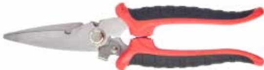
GSE1002 Electronic Scissors Available size: 5 ½" Material: High quality stainless steel Surface: Fine polished Hardness: 54±2 HRC Handle: PP+TPR
