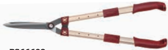
PS66609 Hedge shears Size: 26 3/4" – 32 1/2" Material: 65#MN steel blade Blade thickness: 4.0mm Hardness: 48±2 HRC on blade Surface: sanding polished on blade Handle: telescopic aluminum tube handle with soft PP+TPR grips
