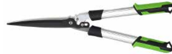
PS76801 Hedge shears Available size: S 675mm Material: 50# high carbon steel blade Surface: Non-stick painted on upper blade, chromed on lower blade Hardness: 46±2HRC Handle: Aluminum tube handle with soft PP+TPR grips
