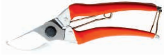
PS33614 Drop forged by-pass pruning shears Available size: 8"(200mm) Material: drop forged stainless steel blade Hardness: 50-52HRC on blade Surface: Fully machine grinding on blade Handle: steel handle with Zinc plated and soft dipped
