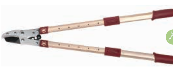
PS66318 Loppers Available size: 27" – 37" Material: upper blade, 65#MN steel, lower blade, 50# high carbon steel Blade thickness: 5.0mm Hardness: 54±2 HRC on blade Surface: Non-stick painting on upper blade, chromed on lower blade Handle: telescopic aluminum tube handle with soft PP+TPR grips
