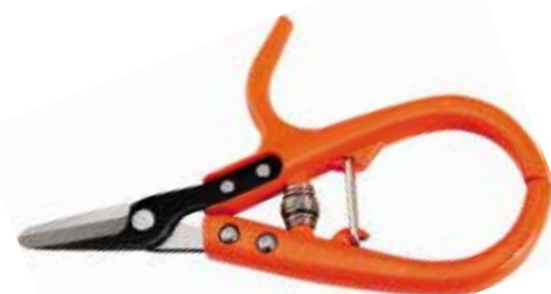
PS27007 Orange shears Available size: 5.5"(135mm) Material: 65#MN steel blade Hardness: 52-54HRC on blade Surface: black finished and fully machine grinding Handle: Zinc alloy handle with powder coated
