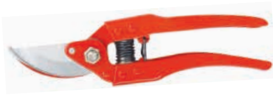
PS33606 Drop forged by-pass pruning shears Available size: 9" (230mm) Material: drop forged 55# high carbon steel body, 65#MN steel changeable blade Hardness: whole-piece heat treatment with hardness 52-54HRC on body, 54-56HRC on changeable blade Surface: fully machine grinding on changeable blade Handle: 45# high carbon steel with red powder coating.
