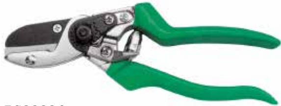
PS83304 Pruning shears Avilable size: 8" (200mm) Material: 65#MN steel blade Hardness: 52-56HRC Surface: non-stick painted on blade Handle: aluminum casting handle with soft dipped
