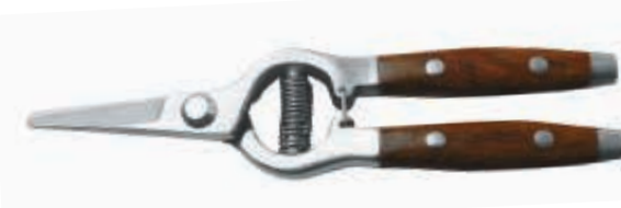
PS41004 Drop Forged pruning shears Available size: 8" Material: whole-piece drop forged stainless steel Hardness: whole-piece heat treatment with hardness 51-53HRC Surface: mirror polished Handle: natural rose wooden with fully polished
