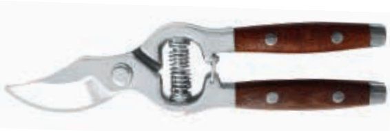
PS41003 Drop Forged by-pass pruning shears Available size: 8" Material: whole-piece drop forged stainless steel Hardness: whole-piece heat treatment with hardness 51-53HRC Surface: mirror polished Handle: natural rose wooden with fully polished
