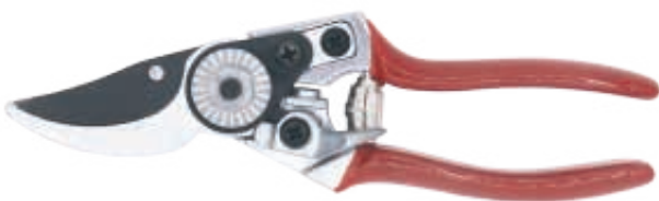
PS113312 Aluminum pruning shears Available size: 7" Material: Aluminum casting body, 65#MN steel blade Hardness: 53±2 HRC on blade Surface: fine polished on aluminum body, Non-stick painted on blade Handle: soft dipped
