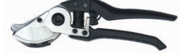
PS33628 Drop forged rose cutter Available size: 8"(200mm) Material: drop forged 55# high carbon steel blade Hardness: 50-54HRC on blade Surface: Fully machine grinding Handle: reinforced nylon
