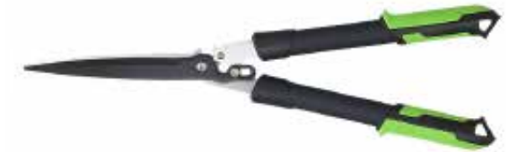
PS76802 Hedge shears Available size: 675mm Material: 50# high carbon steel blade Surface: Non-stick painted on upper blade, chromed on lower blade Hardness: 46±2HRC Handle: Steel tube handle with soft PP+TPR grips
