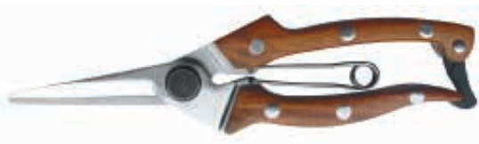
PS41018 Pruning shears Available size: 8" Material: stainless steel Hardness: whole-piece heat treatment with hardness 51-53HRC Surface: Mirror polished Handle: natural rose wooden with fully polished
