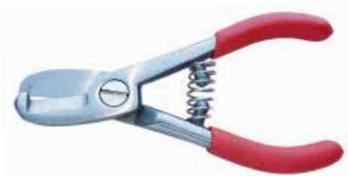
PS27001 Drop forged orange shears Available size: 5.5"(135mm) Material: whole-piece drop forged 55# high carbon steel Hardness: whole-piece heat treatment with hardness 52-54HRC Surface: Fully polished Handle: Soft dipped
