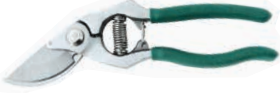
PS33627 Drop forged by-pass pruning shears Available size: 8"(210mm) Material: drop forged 55# high carbon steel body, 65#Mn steel changeable blade Hardness: whole-piece heat treatment with hardness 52-54HRC Surface: fine polished Handle: soft dipped
