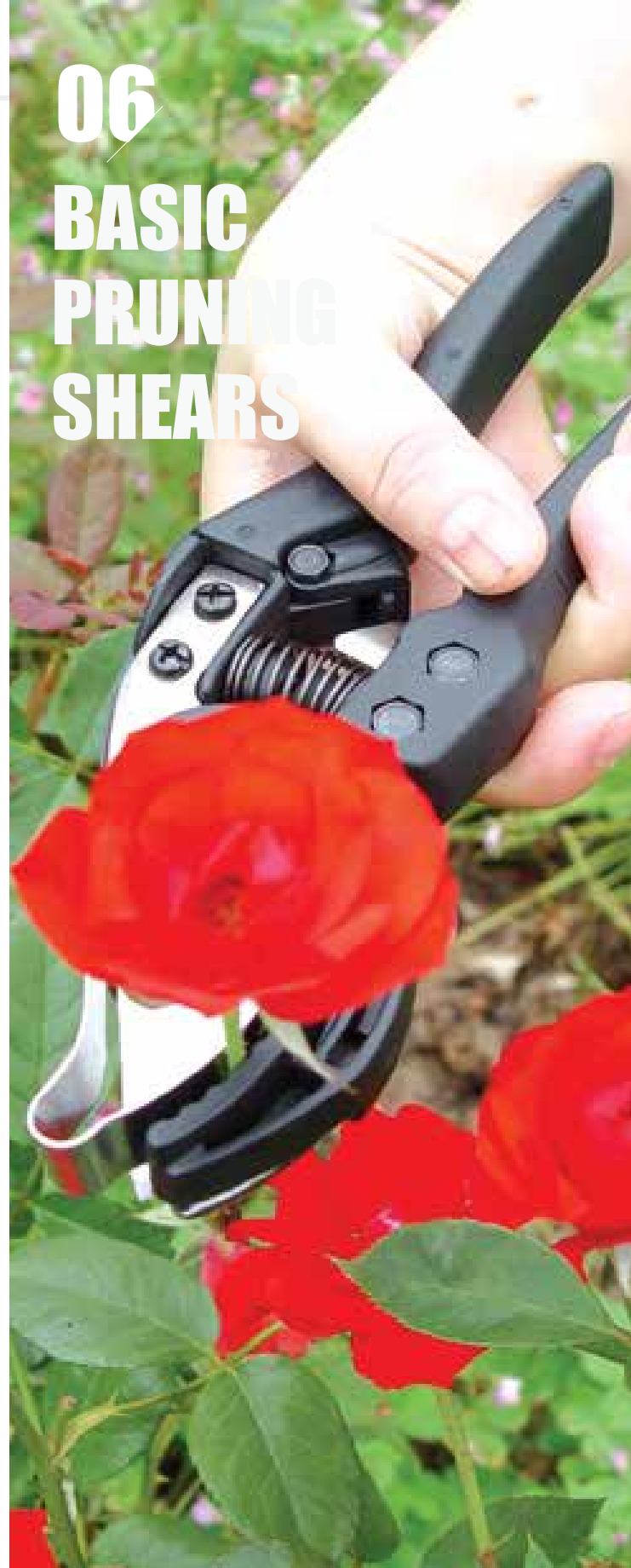
PS83004 Pruning shears Available size: 8" (200mm) Material: 65#MN steel blade Hardness: 52-56HRC Surface: hard chromed Handle: aluminum casting handle with soft TPR grips
