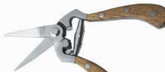
PS41008 Drop Forged pruning shears Available size: 8" Material: drop forged 55# high carbon steel body, 65#MN steel changeable blade Hardness: whole-piece heat treatment with hardness 52-54HRC on body, 54-56HRC on changeable blade Surface: fine polished Handle: ash wooden with fully polished
