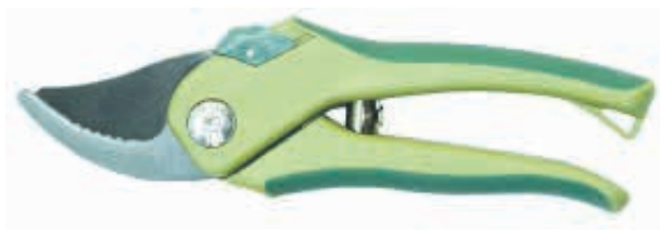
PS8730A Pruning shears Avilable size: 8" (200mm) Material: 65#MN steel blade Hardness: 52-56HRC on blade Surface: non-stick painted on blade Handle: PP+TPR grips
