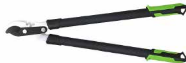
PS66805 Loppers Available size: 750mm Material: 50# high carbon steel blade Surface: Non-stick painted on upper blade, chromed on lower blade Hardness: 52±2HRC Handle: steel tube handle with soft PP+TPR grips
