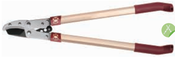
PS66317 Loppers Available size: 27" Material: upper blade, 65#MN steel, lower blade, 50# high carbon steel Blade thickness: 5.0mm Hardness: 54±2 HRC on blade Surface: Non-stick painting on upper blade, chromed on lower blade Handle: aluminum tube handle with soft PP grips
