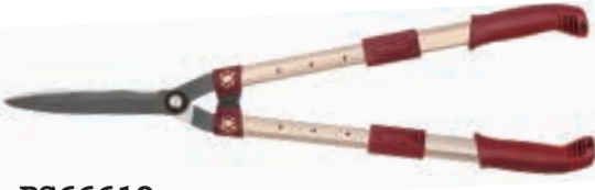
PS66610 Hedge shears Size: 26 3/4" – 32 1/2" Material: 65#MN steel blade Blade thickness: 4.0mm Heat-treatment: 48±2 HRC on blade Surface: sanding polished on blade Handle: telescopic aluminum tube handle with soft PP+TPR grips
