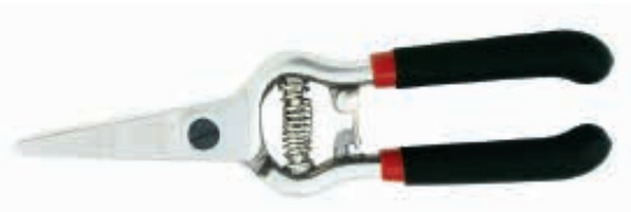
PS33610 Drop forged pruning shears straight blade Available size: 6"(150mm), 8"(200mm) Material: whole-piece drop forged 55# high carbon steel Hardness: whole-piece heat treatment with hardness 50-54HRC Surface: fine polished Handle: soft dipped
