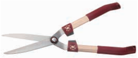
PS66608 Hedge shears Size: 21" Material: 65#MN steel blade Blade thickness: 4.0mm Hardness: 48±2 HRC on blade Surface: fine polished on blade Handle: aluminum tube handle with soft PP grips
