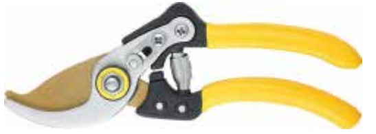
PS83013 Pruning shears Avilable size: 205mm Material: 50# high carbon steel blade Hardness: 52±2 HRC Surface: titanium coated on upper blade, polished on lower blade Handle: Aluminum alloy handle with soft dipped
