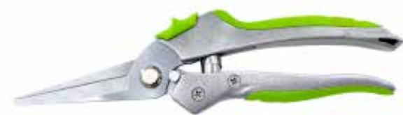
PS89009 Pruning shears Available size: 8" Upper blade: 65#Mn steel, hardness HRC52±2 Lower blade: 65#Mn steel, hardness HRC52±2 Handle: aluminum casting handle with soft TPR grips
