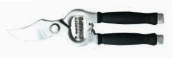
PS33620 Drop forged by-pass pruning shears Available size: 8"(200mm) Material: whole-piece drop forged stainless steel Hardness: whole-piece heat treatment with hardness 50-52HRC Surface: mirror polished Handle: soft TPR grips
