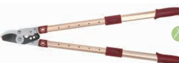
PS66320 Loppers Available size: 27" – 37" Material: upper blade, 65#MN steel, lower blade, 50# high carbon steel Blade thickness: 5.0mm Heat-treatment: 54±2 HRC on blade Surface: Non-stick painting on upper blade, chromed on lower blade Handle: telescopic aluminum tube handle with soft PP+TPR grips
