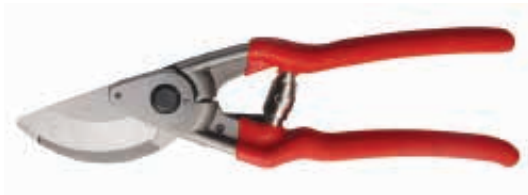
PS33624 Drop forged by-pass pruning shears Available size: 8"(210mm) Material: drop forged 55# high carbon steel body, 65#MN steel changeable blade Hardness: whole-piece heat treatment with hardness 52-54HRC Surface: Fully machine grinding Handle: soft dipped handle
