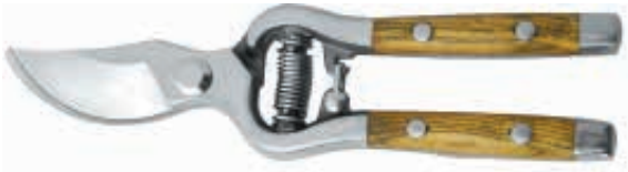
PS40001 Drop Forged by-pass pruning shears Available size: 7", 8" Material: whole-piece drop forged stainless steel Hardness: whole-piece heat treatment with hardness 51-53HRC Surface: mirror polished Handle: ash wooden with fully polished
