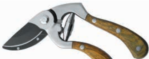
PS41007 Drop Forged by-pass pruning shears Available size: 7" 8" Material: drop forged 55# high carbon steel body, 65#MN steel changeable blade Hardness: whole-piece heat treatment with hardness 52-54HRC on body, 54-56HRC on changeable blade Surface: non-stick painted on changeable blade Handle: ash wooden with fully polished
