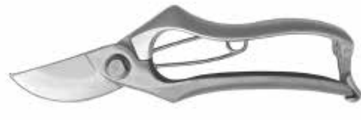
PS33616 Drop forged by-pass pruning shears Available size: 8"(200mm) Material: whole-piece drop forged stainless steel Hardness: whole-piece heat treatment with hardness 50-52HRC Surface: Scallop machine grinding and mirror polished on blade Handle: fine polished
