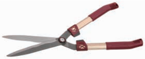
PS66607 Hedge shears Size: 22" Material: 65#MN steel blade Blade thickness: 4.0mm Hardness: 48±2 HRC on blade Surface: sanding polished on blade Handle: aluminum tube handle with soft PP grips
