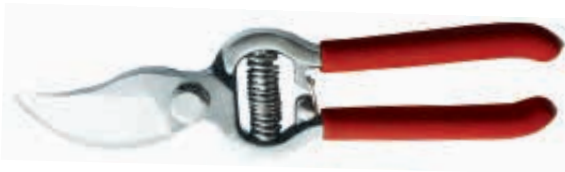
PS33607 Drop forged by-pass pruning shears Available size: 8"(200mm) Material: whole-piece drop forged Chrome-vanadium steel Hardness: whole-piece heat treatment with hardness 52-54HRC Surface: fully machine grinding Handle: soft dipped
