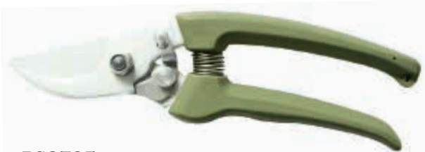
PS8735 Pruning shears Avilable size: 7"(190mm) Material: 65#MN steel blade Hardness: 54-56HRC Surface: chromed Handle: PP grips
