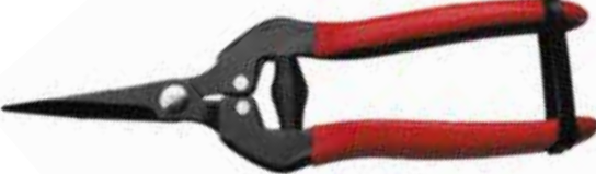
PS27004B Fruit shear straight/curved blade Available size: 7" Material: 65#MN steel blade Hardness: 52-54HRC on blade Surface: black finished on blade Handle: 45# high carbon steel and soft dipped
