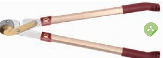
PS66309 Loppers Available size: 27" Material: upper blade, 65#MN steel lower blade, 50# high carbon steel Blade thickness: 5.0mm Hardness: 54±2 HRC on blade Surface: titanium coated on upper blade, chromed on lower blade Handle: aluminum tube handle with soft PP grips
