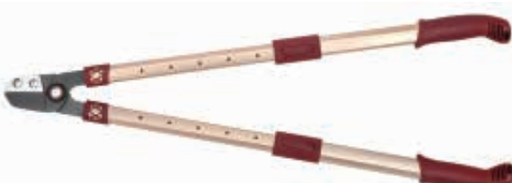
PS66306 Loppers Available size: 24 3/4" – 34 3/4" Material: upper blade, 65#MN steel lower blade, 50# high carbon steel Blade thickness: 5.0mm Hardness: 54±2 HRC on blade Surface: Non-stick painting on blade Handle: telescopic aluminum tube handle with soft PP+TPR grips
