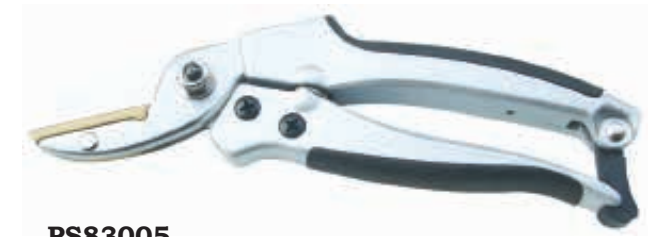
PS83005 Pruning shears Available size: 8" (200mm) Material: 65#MN steel blade Hardness: 52-56HRC Surface: hard chromed Handle: aluminum casting handle with soft TPR grips
