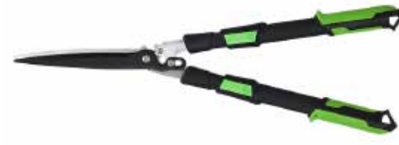
PS76803 Hedge shears Available size: 750mm-950mm Material: 50# high carbon steel blade Surface: Non-stick painted on upper blade, chromed on lower blade Hardness: 46±2HRC Handle: Telescopic steel tube handle with soft PP+TPR grips
