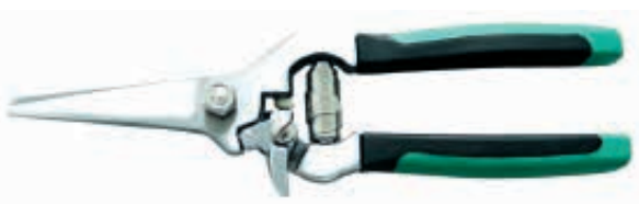
PS33622 Drop forged pruning shears Available size: 8"(200mm) Material: whole-piece drop forged 55# high carbon steel Hardness: whole-piece heat treatment with hardness 52-54HRC Surface: fine polished Handle: Twin-color soft TPR grips
