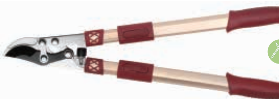
PS66316 Loppers Available size: 27" – 37" Material: upper blade, 65#MN steel, lower blade, 50# high carbon steel Blade thickness: 5.0mm Hardness: 54±2 HRC on blade Surface: Non-stick painting on upper blade, chromed on lower blade Handle: telescopic aluminum tube handle with soft PP+TPR grips
