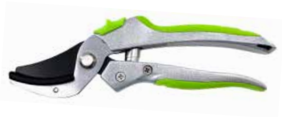
PS89007 Pruning shears Available size: 8" Upper blade: 65#Mn steel blade with non-stick painted, hardness HRC54±2 Lower blade: 50# high carbon steel with chromed, hardness HRC46±2 Handle: aluminum casting handle with soft TPR grips
