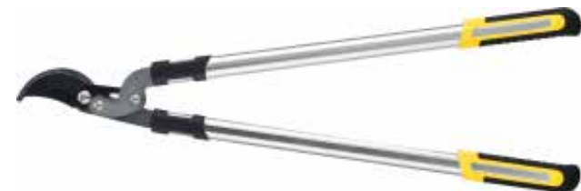
PS63004 Loppers Available size: 30 1/2" Material: 50# high carbon steel blade Hardness: 52±2 HRC Surface: Non-stick painting on upper blade, Chromed on lower blade Handle: Aluminum tube handle with soft PP+TPR grips
