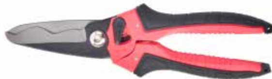
GSE1010 Electronic Scissors Available size: 8 ½" Material: High quality stainless steel Surface: Fine polished Hardness: 54±2 HRC Handle: PP+TPR
