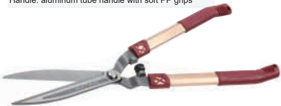
PS66602 Drop forged hedge shears Size: 23 3/4" Material: drop forged 55# high carbon steel blade Blade thickness: 5.5mm Hardness: 52±2 HRC on blade Surface: fully machine grinding Handle: aluminum tube handle with soft PP grips
