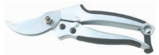
PS83004 Pruning shears Available size: 8" (200mm) Material: 65#MN steel blade Hardness: 52-56HRC Surface: hard chromed Handle: aluminum casting handle with soft TPR grips
