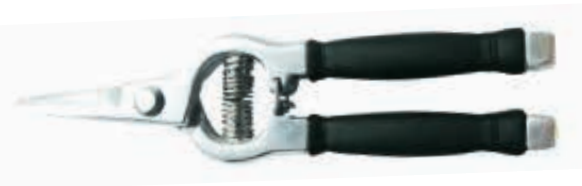
PS33621 Drop forged pruning shears Available size: 8"(200mm) Material: whole-piece drop forged stainless steel Hardness: whole-piece heat treatment with hardness 50-52HRC Surface: mirror polished Handle: soft TPR grips
