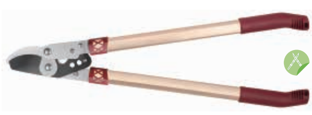
PS66319 Loppers Available size: 27" Material: upper blade, 65#MN steel, lower blade, 50# high carbon steel Blade thickness: 5.0mm Hardness: 54±2 HRC on blade Surface: Non-stick painting on upper blade, chromed on lower blade Handle: aluminum tube handle with soft PP grips
