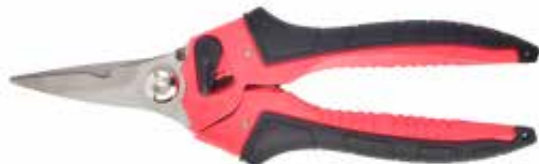
GSE1007 Electronic Scissors Available size: 8" Material: High quality stainless steel Surface: Fine polished Hardness: 54±2 HRC Handle: PP+TPR
