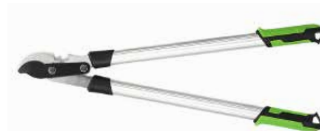
PS66801 Loppers Available size: 750mm Material: 50# high carbon steel blade Surface: Non-stick painted on upper blade, chromed on lower blade Hardness: 52±2HRC Handle: Aluminum tube handle with soft PP+TPR grips
