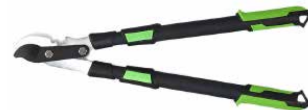
PS66807 Loppers Available size: 685mm-935mm Material: 50# high carbon steel blade Surface: Non-stick painted on upper blade, chromed on lower blade Hardness: 52±2HRC Handle: Telescopic steel tube handle with soft PP+TPR grips
