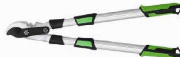
PS66803 Loppers Available size: 705mm-955mm Material: 50# high carbon steel blade Surface: Non-stick painted on upper blade, chromed on lower blade Hardness: 52±2HRC Handle: Telescopic aluminum tube handle with soft PP+TPR grips
