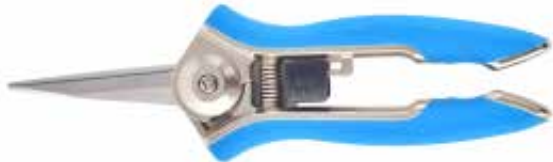
PS86002 Pruning shears Available size: 6" Material: stainless steel Hardness: 52-56HRC Surface: fine polished Handle: zinc alloy and soft TPR grips
