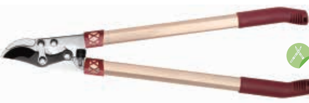
PS66315 Loppers Available size: 27" Material: upper blade, 65#MN steel, lower blade, 50# high carbon steel Blade thickness: 5.0mm Hardness: 54±2 HRC on blade Surface: Non-stick painting on upper blade, chromed on lower blade Handle: aluminum tube handle with soft PP grips
