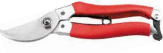
PS33615 By-pass pruning shears Available size: 8"(200mm) Material: 65#MN steel Hardness: 54-56HRC on blade Surface: Scallop machine grinding on blade Handle: 45# high carbon steel with metallic lacquered and soft dipped
