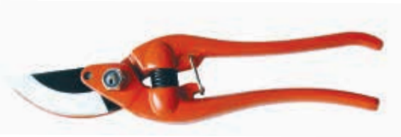
PS33604 Drop forged by-pass pruning shears Available size: 8"(200mm), 9"(230mm) Material: drop forged 55# high carbon steel body, 65#MN steel changeable blade Hardness: whole-piece heat treatment with hardness 52-54HRC on body, 54-56HRC on changeable blade Surface: Black finished on changeable blade Handle: red powder coated
