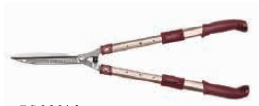
PS66614 Hedge shears Total Size: 27 1/2"-33 1/2" Available blade size: 9 1/2" Material: drop forged 55# high carbon steel blade Blade thickness: 5.5mm Hardness: 52±2 HRC Surface: fully machine grinding Handle: Telescopic aluminum tube handle with soft PP grips
