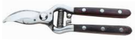
PS41009 Drop Forged by-pass pruning shears Available size: 8 1/2" Material: drop forged stainless steel body, stainless steel blade Hardness: whole-piece heat treatment with hardness 51-53HRC on body, 52-54HRC on changeable blade Surface: fine polished Handle: wooden with fully polished
