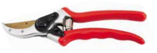
PS113304T Drop forged aluminum pruning shears Available size: 8" (210mm) Material: drop forged aluminum body, SK-5 steel blade Hardness: 54-56HRC on blade Surface: oxidation treatment on aluminum body, titanium coated on blade Handle: soft dipped
