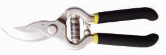
PS33613 Drop forged by-pass pruning shears Available size: 8 1/2"(220mm) Material: drop forged 55# high carbon steel body, 65#MN steel changeable blade Hardness: whole-piece heat treatment with hardness 52-54HRC Surface: fine polished Handle: soft dipped
