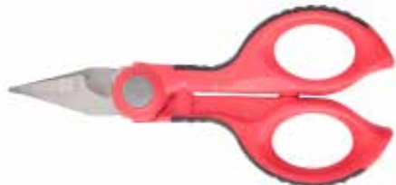
GSE1002 Electronic Scissors Available size: 5 ½" Material: High quality stainless steel Surface: Fine polished Hardness: 54±2 HRC Handle: PP+TPR
