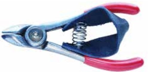
PS27006 Drop forged orange shears Available size: 4.5"(115mm), 5.5"(140mm) Material: whole-piece drop forged 55# high carbon steel Hardness: whole-piece heat treatment with hardness 52-54HRC Surface: Fully vibration rubbing Handle: Soft dipped
