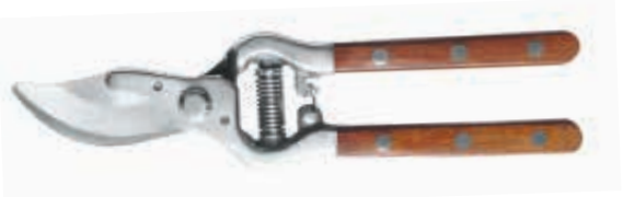
PS41014 Drop forged by-pass pruning shears Avilable size: 8 1/2" Material: drop forged stainless steel body, stainless steel changeable blade Hardness: whole-piece heat treatment with hardness 51-53HRC on body, 52-54HRC on changeable blade Surface: Fine polished Handle: wooden handle with fully polished
