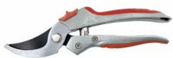
PS89008 Pruning shears Available size: 8" Upper blade: 65#Mn steel blade with non-stick painted, hardness HRC54±2 Lower blade: 50# high carbon steel with chromed, hardness HRC46±2 Handle: aluminum casting handle with soft TPR grips
