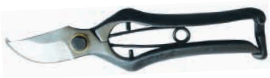
PS33619 Drop forged Pruning Shears Available size: 8" (200mm) Material: whole-piece drop forged 55# high carbon steel Hardness: whole-piece heat treatment with hardness 52-54HRC Surface: Fully machine grinding Handle: black finished
