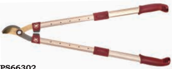
PS66302 Loppers Available size: 25 1/2" - 35 1/2" Material: upper blade, 65#MN steel lower blade, 50# high carbon steel Blade thickness: 5.0mm Hardness: 54±2 HRC on blade Surface: titanium coated on upper blade, Non-stick painting on lower blade Handle: telescopic aluminum tube handle with soft PP+TPR grips
