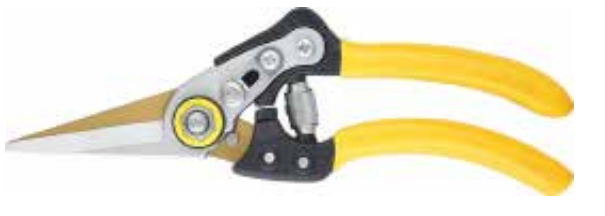
PS83015 Pruning shear Avilable size: 215mm Material: 50# high carbon steel blade Hardness: 52±2 HRC Surface: titanium coated on upper blade, polished on lower blade Handle: Aluminum alloy handle with soft dipped
