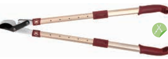
PS66312 Loppers Available size: 26 3/4" – 34 3/4" Material: upper blade, 65#MN steel, lower blade, 50# high carbon steel Blade thickness: 5.0mm Hardness: 54±2 HRC on blade Surface: Non-stick painting on upper blade, chromed on lower blade Handle: telescopic aluminum tube handle with soft PP+TPR grips
