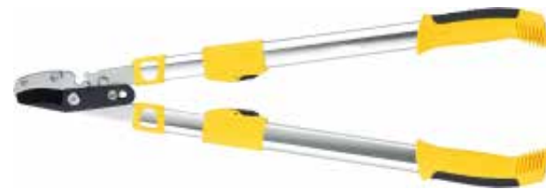
PS63006 Loppers Available size: 29" - 39" Material: 50# high carbon steel blade Hardness: 52±2 HRC Surface: Non-stick painting on upper blade, Chromed on lower blade Handle: Telescopic aluminum tube handle with soft PP+TPR grips
