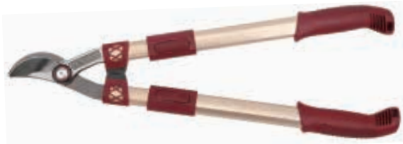
PS66304 Drop Forged Loppers Available size: 25 1/2" – 35 1/2" Material: drop forged 55# high carbon steel blade Blade thickness: 7.0mm Hardness: 54±2 HRC on blade Surface: fully machine grinding Handle: telescopic aluminum tube handle with soft PP+TPR grips
