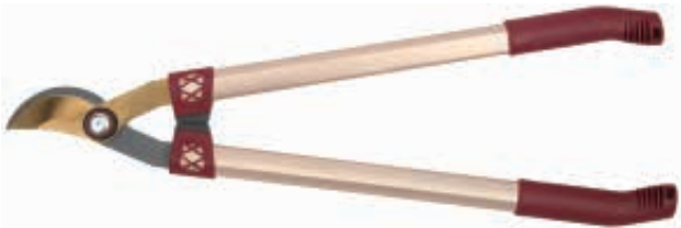
PS66301 Loppers Available size: 25 1/2" Material: upper blade, 65#MN steel lower blade, 50# high carbon steel Blade thickness: 5.0mm Hardness: 54±2 HRC on blade Surface: titanium coated on upper blade, Non-stick painting on lower blade Handle: aluminum tube handle with soft PP grips
