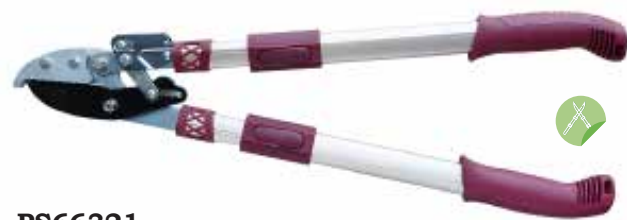
PS66321 Loppers Available size: 27 1/4" -37" Blade size: 4" Material: Upper blade: 65#MN steel, Lower blade: 50# high carbon steel Blade thickness: 5mm Hardness: 52±2 HRC Surface: Non-stick painting on upper blade, Chromed on lower blade Handle: Telescopic aluminum tube handle with soft PP grips
