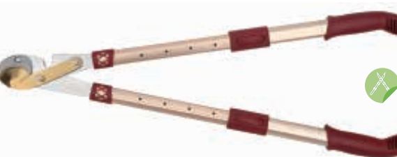
PS66310 Loppers Available size: 27" – 32 3/4" Material: upper blade, 65#MN steel, lower blade, 50# high carbon steel Blade thickness: 5.0mm Hardness: 54±2 HRC on blade Surface: titanium coated on upper blade, chromed on lower blade Handle: telescopic aluminum tube handle with soft PP+TPR grips
