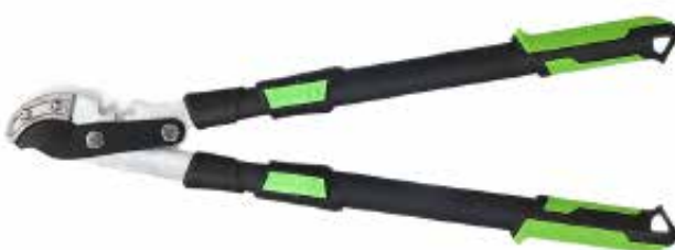
PS66808 Loppers Available size: 685mm-935mm Material: 50# high carbon steel blade Surface: Non-stick painted on upper blade, chromed on lower blade Hardness: 52±2HRC Handle: Telescopic steel tube handle with soft PP+TPR grips
