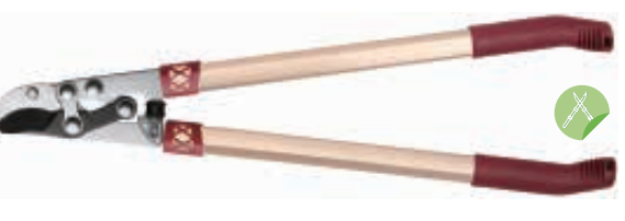
PS66313 Loppers Available size: 27" Material: upper blade, 65#MN steel, lower blade, 50# high carbon steel Blade thickness: 5.0mm Hardness: 54±2 HRC on blade Surface: Non-stick painting on upper blade, chromed on lower blade Handle: aluminum tube handle with soft PP grips
