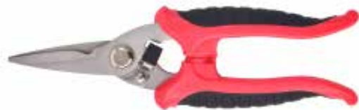
GSE1003 Electronic Scissors Available size: 7" Material: High quality stainless steel Surface: Fine polished Hardness: 54±2 HRC Handle: PP+TPR
