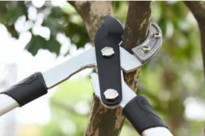
PS66319 Loppers Available size: 27" Material: upper blade, 65#MN steel, lower blade, 50# high carbon steel Blade thickness: 5.0mm Hardness: 54±2 HRC on blade Surface: Non-stick painting on upper blade, chromed on lower blade Handle: aluminum tube handle with soft PP grips
