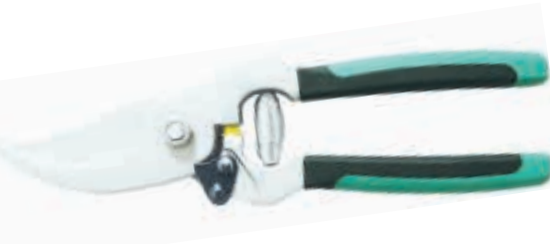
PS33623 Drop forged by-pass pruning shears Available size: 8"(200mm) Material: whole-piece drop forged 55# high carbon steel Hardness: whole-piece heat treatment with hardness 52-54HRC Surface: fine polished Handle: Twin-color soft TPR grips
