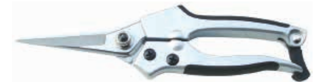
PS83003 Pruning shears Available size: 8" (200mm) Material: 65#MN steel blade Hardness: 52-56HRC Surface: hard chromed Handle: aluminum casting handle with soft TPR grips
