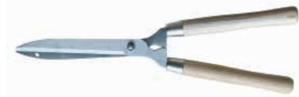
PS72005 Hedge shears Size: 21" Material: 50# high carbon steel Hardness: 48-52HRC Surface: fine polished Handle: ash wooden with fully polished
