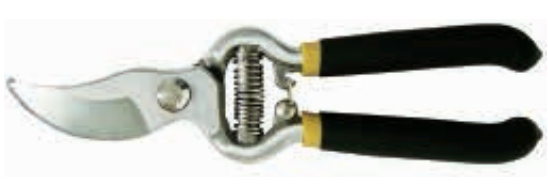
PS33609 Drop forged by-pass pruning shears Available size: 8"(200mm) Material: whole-piece drop forged 55# high carbon steel Hardness: whole-piece heat treatment with hardness 52-54HRC Surface: fine polished
