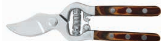
PS41006 Drop Forged by-pass pruning shear Available size: 8" Material: whole-piece drop forged stainless steel Hardness: whole-piece heat treatment with hardness 51-53HRC Surface: mirror polished Handle: wooden with fully polished
