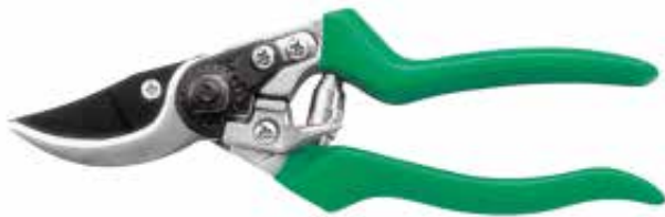
PS83305 Pruning shears Avilable size: 8" (200mm) Material: 65#MN steel blade Hardness: 52-56HRC Surface: non-stick painted on blade Handle: aluminum casting handle with soft dipped
