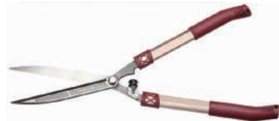
PS66613 Hedge shears Total Size: 25" Available blade size: 9 1/2" Material: drop forged 55# high carbon steel blade Blade thickness: 5.5mm Hardness: 52±2 HRC Surface: fully machine grinding Handle: aluminum tube handle with soft PP grips
