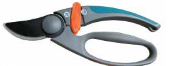
PS83002 Pruning shears Avilable size: 8" Material: 65#MN steel blade Hardness: 52±2 HRC Surface: non-stick painting on upper blade, chromed on lower blade Handle: Soft PP+TPR handles
