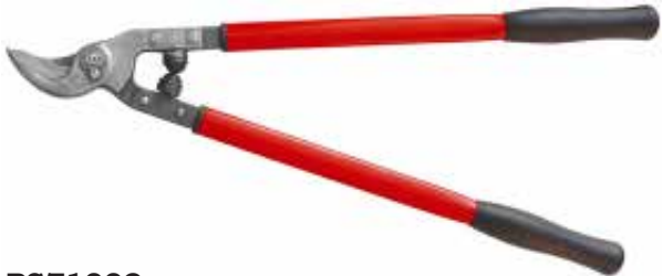
PS71002 Drop forged loppers Available size: 23" Material: drop forged 55# high carbon steel Hardness: 52-54HRC on blade Surface: fine polished Handle: steel tube handle with red powder coated+PP grips
