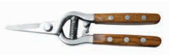
PS41012 Drop Forged pruning shears Available size: 8" Material: whole-piece drop forged stainless steel Hardness: whole-piece heat treatment with hardness 51-53HRC Surface: mirror polished Handle: ash wooden with fully polished
