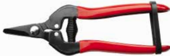
PS27004 Fruit shears curved blade Available size: 6 1/2", 7" Material: 65#MN steel blade Hardness: 52-56HRC on blade Surface: black finished Handle: 45# high carbon steel and soft dipped
