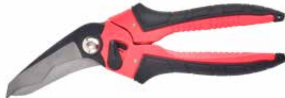
GSE1009 Electronic Scissors Available size: 8 ½" Material: High quality stainless steel Surface: Fine polished Hardness: 54±2 HRC Handle: PP+TPR
