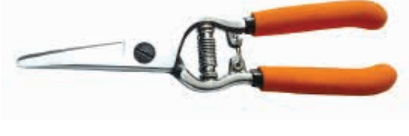
PS33611 Drop forged pruning shears curved blade Available size: 6"(150mm), 8"(200mm) Material: whole-piece drop forged 55# high carbon steel Hardness: whole-piece heat treatment with hardness 50-54HRC Surface: fine polished Handle: soft dipped
