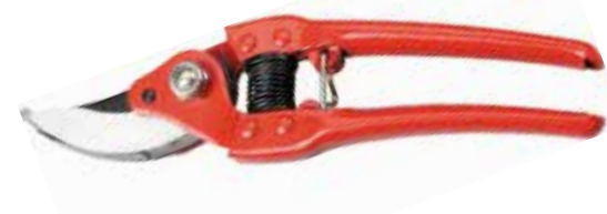
PS33606A Drop forged by-pass pruning shears Available size: 9" (230mm) Material: drop forged 55# high carbon steel body, 65#MN steel changeable blade Hardness: whole-piece heat treatment with hardness 52-54HRC on body, 54-56HRC on changeable blade Surface: black finished and fully machine grinding on changeable blade Handle: 45# high carbon steel with red powder coating.
