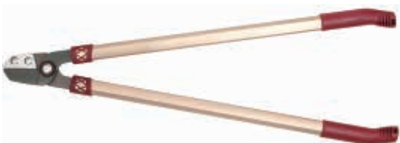
PS66305 Loppers Available size: 24 3/4" Material: upper blade, 65#MN steel lower blade, 50# high carbon steel Blade thickness: 5.0mm Hardness: 54±2 HRC on blade Surface: Non-stick painting on blade Handle: aluminum tube handle with soft PP grips
