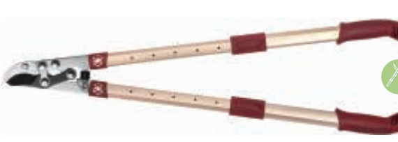
PS66314 Loppers Available size: 27" – 37" Material: upper blade, 65#MN steel, lower blade, 50# high carbon steel Blade thickness: 5.0mm Hardness: 54±2 HRC on blade Surface: Non-stick painting on upper blade, chromed on lower blade Handle: telescopic aluminum tube handle with soft PP+TPR grips
