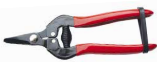
PS27004A Fruit shears straight blade Available size: 6 1/2", 7" Material: 65#MN steel blade Hardness: 52-56HRC on blade Surface: black finished Handle: 45# high carbon steel and soft dipped
