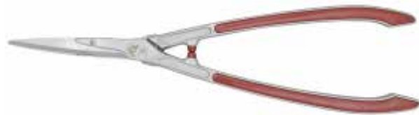
PS66611 Hedge shears Total Size: 26" Available blade size: 8", 9", 10" Material: 65#MN steel blade Blade thickness: 4mm Hardness: 52±2 HRC Surface: Chromed Handle: Aluminum handle with soft PP grips
