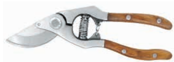
PS41010 Drop Forged by-pass pruning shears Available size: 8 1/2" Material: drop forged stainless steel body, stainless steel blade Hardness: whole-piece heat treatment with hardness 51-53HRC on body, 52-54HRC on changeable blade Surface: fine polished Handle: wooden with fully polished
