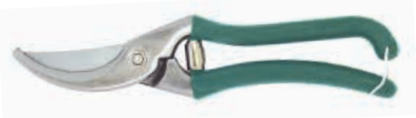
PS33625 Drop forged by-pass pruning shears Available size: 8"(200mm) Material: whole-piece drop forged 55# high carbon steel Hardness: whole-piece heat treatment with hardness 52-54HRC Surface: fine polished Handle: soft dipped
