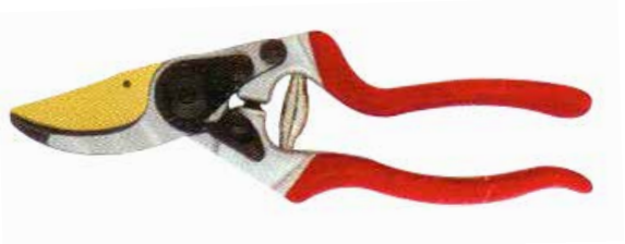
PS113303T Drop forged aluminum pruning shears Available size: 8" (210mm) Material: Drop forged aluminum body, SK-5 steel blade Hardness: 54-56HRC on blade Surface: oxidation treatment on aluminum body, titanium coated on blade Handle: soft dipped
