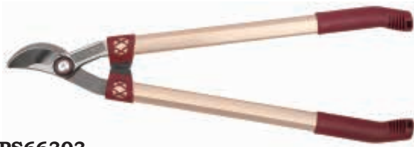
PS66303 Drop Forged Loppers Available size: 25 1/2" Material: drop forged 55# high carbon steel blade Blade thickness: 7.0mm Hardness: 54±2 HRC on blade Surface: fully machine grinding Handle: aluminum tube handle with soft PP grips
