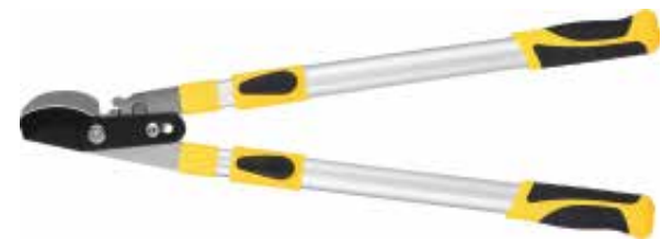
PS63005 Loppers Available size: 26 1/2" -39 1/2" Material: 50# high carbon steel blade Hardness: 52±2 HRC Surface: Non-stick painting on upper blade, Chromed on lower blade Handle: Telescopic aluminum tube handle with soft PP+TPR grips
