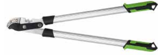
PS66802 Loppers Available size: 750mm Material: 50# high carbon steel blade Surface: Non-stick painted on upper blade, chromed on lower blade Hardness: 52±2HRC Handle: Aluminum tube handle with soft PP+TPR grips
