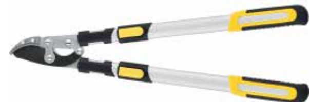
PS63003 Loppers Available size: 28 1/2" -35 1/2" Material: 50# high carbon steel blade Hardness: 52±2 HRC Surface: Non-stick painting on upper blade, Chromed on lower blade Handle: Telescopic T shape aluminum tube handle with soft PP+TPR grips
