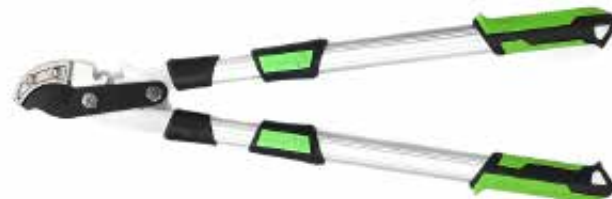
PS66804 Loppers Available size: 705mm-955mm Material: 50# high carbon steel blade Surface: Non-stick painted on upper blade, chromed on lower blade Hardness: 52±2HRC Handle: Telescopic aluminum tube handle with soft PP+TPR grips
